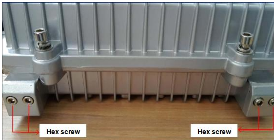
Figure: Unscrew the hex screw at the bottom of the EOC Master
